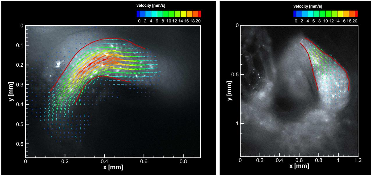
Figure 4: PIV measurement in the ventricle (left) and in the atrium (right) of a chicken embryo.
