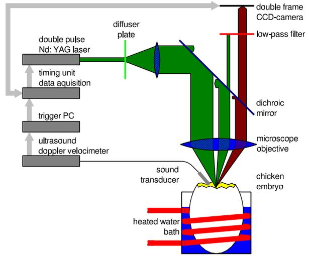
Figure 2: A  $\mu$ PIV set-up, using fluorescent stealth liposomes as tracer particles.
