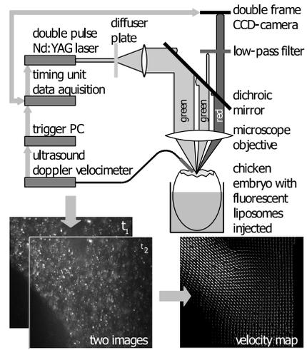
Figure 2: The  $\mu$ PIV set-up, using a fluorescence microscope.
