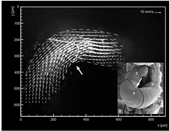
Figure 3: PIV measurement in the developing ventricle of a normal Hamburger and Hamilton stage 15 chicken embryo. The location and spatial orientation of the measurement plane relative to the looping heart is indicated in the scanning electron micrographs from Männer (2000).
