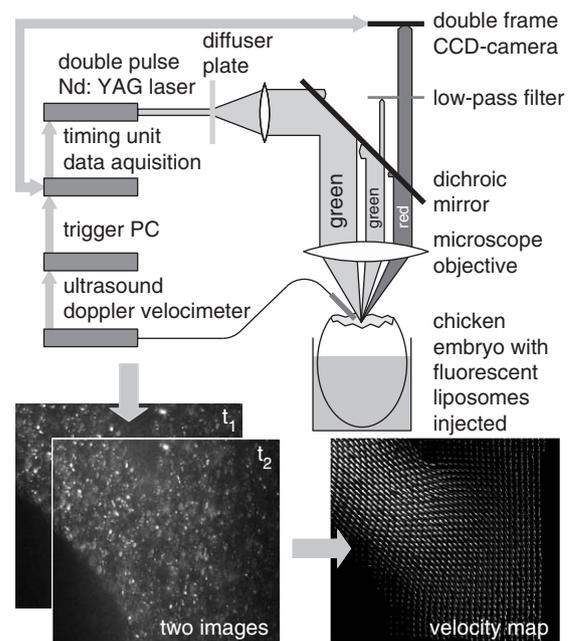
Fig. 2.  $\mu$ PIV set-up, using a fluorescence microscope. A dichroic mirror and a low-pass filter allow only the light emitted by the fluorescent tracer particles to reach the camera.
