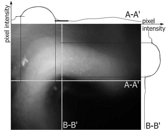
Fig. 5. The average of 100 image frames reveals the inner lumen boundary as a bright region. Due to the approximately circular cross-section of the vessel, the theoretical grey value intensity function has an elliptical shape. The intersection point of the theoretical intensity profile (least square fit to the data) and the grey level offset of the neighboring region accurately defines the position of the vessel wall.
