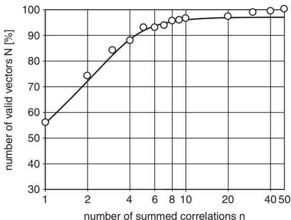
Fig. 4. Percentage of reliable vectors as a function of the number of summed correlation functions. If interrogation areas of  $64 \times 64$  pixels are used, 50 image pairs are sufficient to obtain close to 100% reliable vectors.
